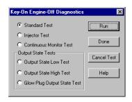
The content of this dialog box is dependent on the engine electronics platform. Confirm the engine electronics platform by looking at the MD main window's title bar. You must exit MD in order to change the engine electronics platform.
