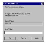
After modifying the "Tire Revs" value, MD will display other dialog boxes prompting you to update the affected parameters. MD will also calculate the appropriate value for the affected parameter based on the new special programmable parameter's value. For example, "Low Axle Ratio Pulses Per Mile" is an affected parameter when you change "Tire Revs".
