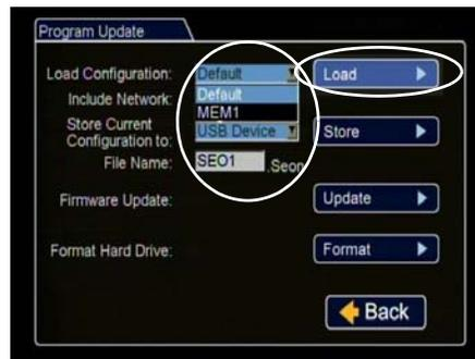
**Figure 3-3** Loading USB Configuration
