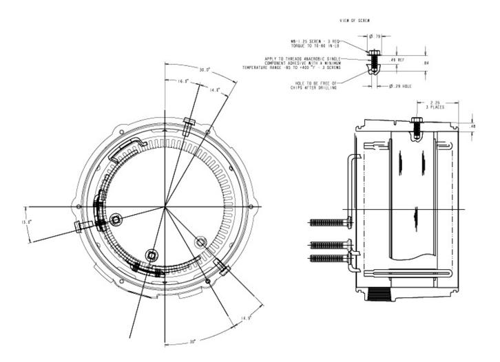
Figure 2 (Detail – Stator Locking Process)
